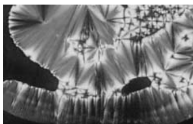
Figure 3. Focal-conic smectic texture of guanidinium octylbenzenesulfonate at 184 °C.
